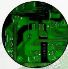
FR4 2,00 mm 70 µCu 4 Katmanlı / Layer Yeşil/Green Solder Mask Beyaz/White Silkscreen HAL Leadfree
