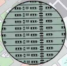
Alüminyum 1,60 mm 0/35 µCu Beyaz/White Solder Mask Siyah/Black Silkscreen V-Cut HAL Leadfree
